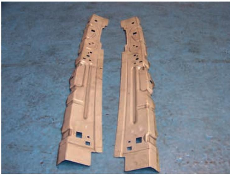
Prototype cold stamped windshield pillars after cutting and painting
