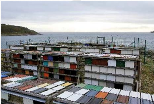
ArcelorMittal's weathering site in Brest (France) is managed by the French Institute of Corrosion © ArcelorMittal
