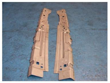
Prototype cold stamped windshield pillars after cutting and painting
