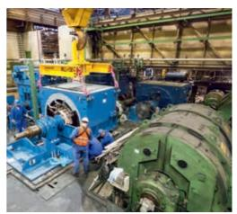
Assembly of the new synchronous motor for the cold strip tandem mill (left) and an old direct current motor (right).
