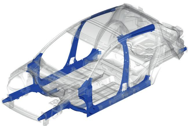
HF1050 can already be utilised to create structural components of the BIW.
