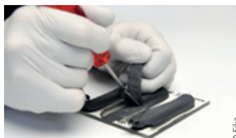
Adhesion tests carried out by Sika showed adhesives used with Magnelis® substrates were unaffected by long-term ageing conditions.
