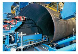
Pipes undergoing helical submerged arc welding (HSAW) at CPW.
