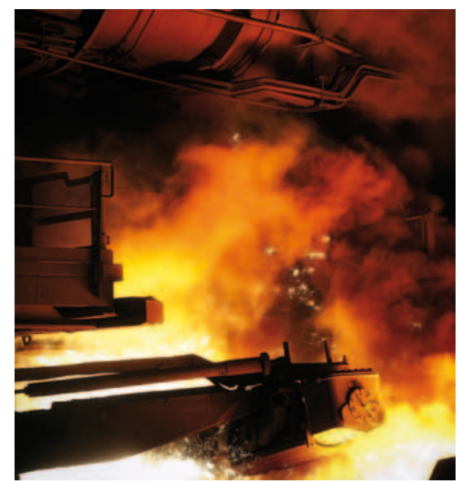
Fos-sur-Mer performs a double desulphurisation and Si-Ca treatment. HIC-resistant steels have been produced there for 20 years.
